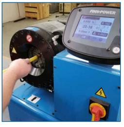
Our press adjusts to the final-compressed outside dimension as designated by each cable and ferrule manufacturer. Statistics are available for each crimp.
